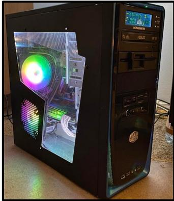
Will Pitts proudly presented his new build. This is a modern Windows 11 computer based on the Gigabyte GA-H57M-USB 3.0 motherboard, equipped with a Core i7 870, 8GB RAM, 128GB SSD and a 1TB hard drive. This motherboard has the unique ability to support one floppy, so Will decided to incorporate a 5.25" drive. His objective, years in the making, was to have a modern build with a 5.25" floppy drive. Congratulations to Will! He mentions that his next project is connecting an 8" floppy drive.
