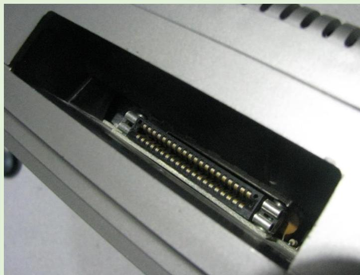
In the above image, the cart's connector is easily seen because the flap was pushed open and it stayed in this position, even without a cartridge.
