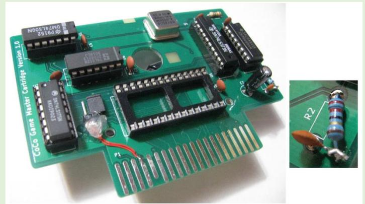
To prevent the CoCo from executing non-existing ROM code, I decided to jumper pins 7 (Q) and 8 (CART\*). The image of the assembled GMC shows the header and jumper. This image also shows how I added the capacitor to bring the GMC to version 2.
