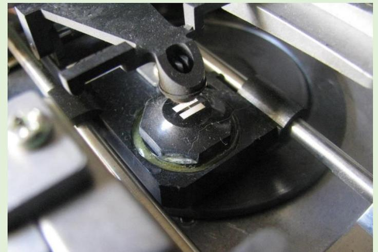
Yup, that's the head, the thingy that looks like a “pause” symbol. Carefully, with a Q-tip and some alcohol, I cleaned the head. After that was done, I reassembled the floppy drive. For me, that was the last activity that I could perform on the drive. I hooked everything up and retested. No change.
