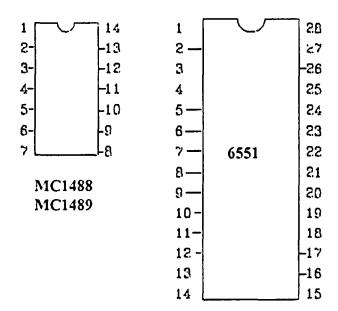
Now, piggyback the 1488 to the original on the board and do the same with the 1489. Solder only the pins you left pointing down at this time.
